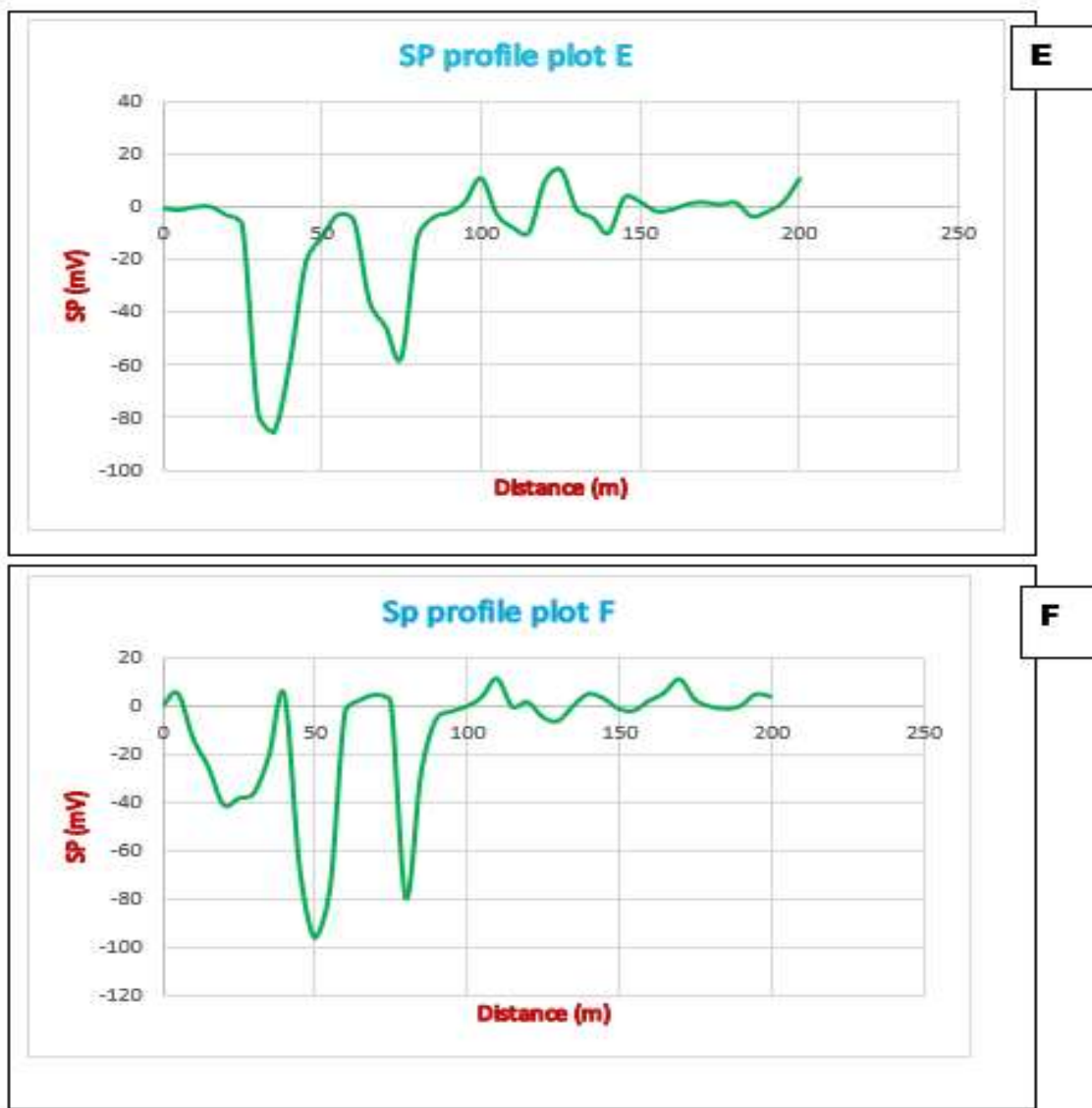
Figure 10: Self-potential profile plots for E and F
